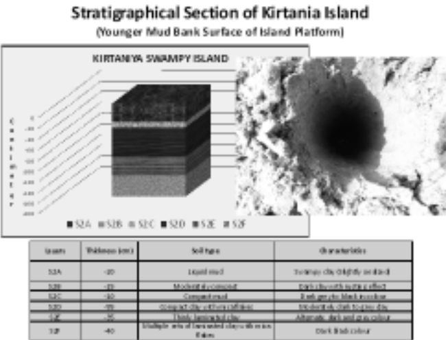
Figure 3 Stratigraphical Section of Kirtania Island and Associated Sediment Characters
