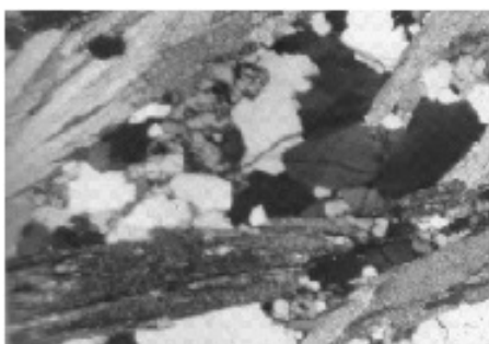
Well developed gneissosity formed by muscovite and quartz-feldspathic minerals. (Under Crossed Nicols, 40x)
