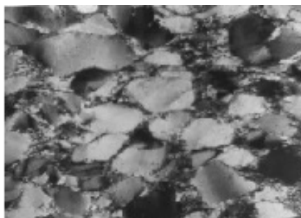
Quartz-feldspar (Schist), pressure effect is evident from the undulose surface of Biotite and quartz grains. (Under Crossed Nicols, 40x)
