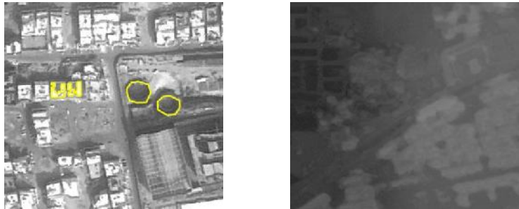
Figure 3. (a) Orthophoto [Digitized] (b) Final DSM over Digitized region
