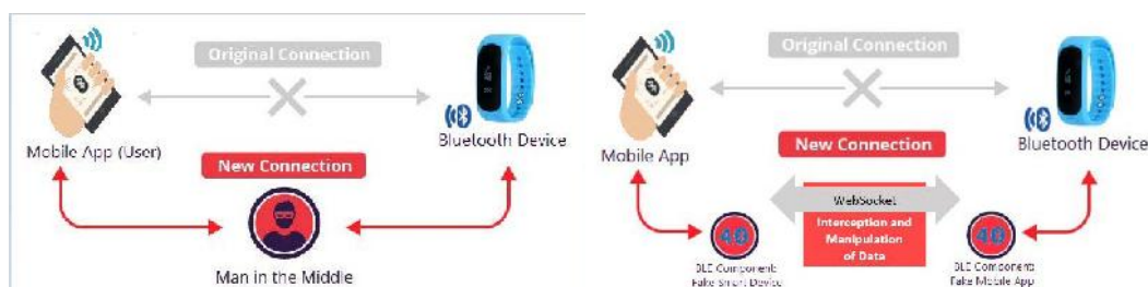
Figure 6. Man in the middle attack in a normal sensor and a BLE sensor
