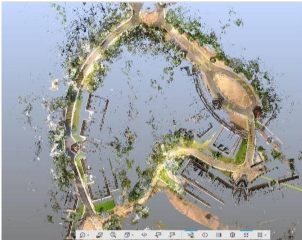
Figure 3. Top view of the registered, geo-referenced and colored scans
