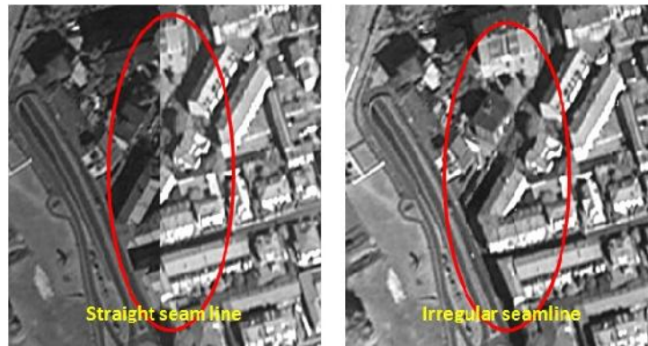
Figure 9. Mosaic of two images with straight seam line and irregular seam line
