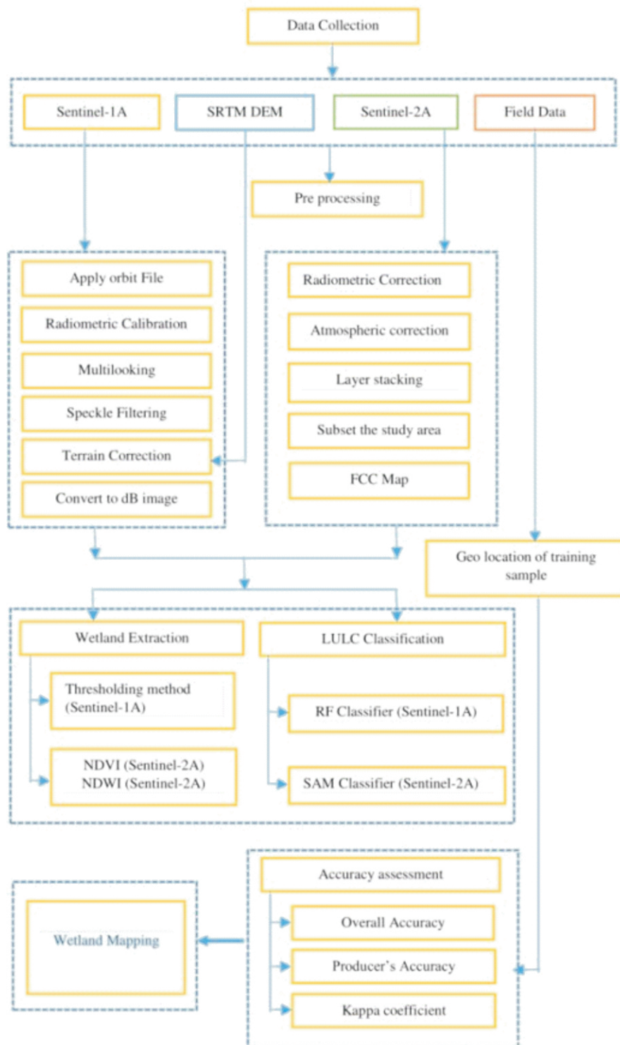
Fig.3 Detailed methodological flowchart for wetland mapping
