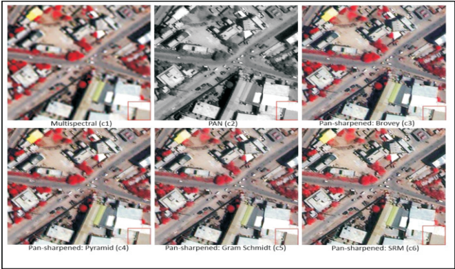
Fig.4 Input (c1 and c2) and Output Pan-sharpened images (c4, c4, c5, c6) of Cartosat-2S data
